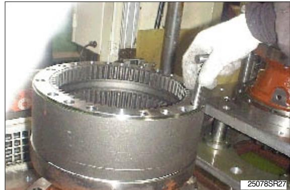
Assemble ring gear with case by screwing socket bolt(M16) (24).
