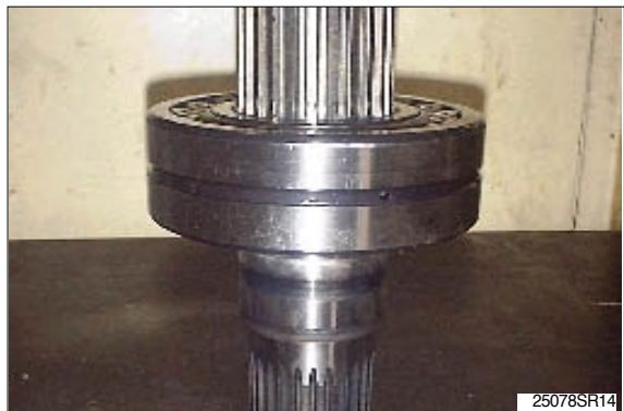
Turn the drive shaft(2) to have the 2 tap hole side down and inject grease oil into roller bearing(4).
