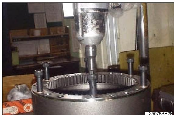
Move out No.1 sun gear(17) and No.1 carrier sub assy by using jig.
