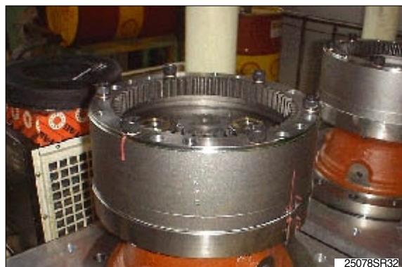
Full out No.2 carrier sub assy by using jig and crane.
