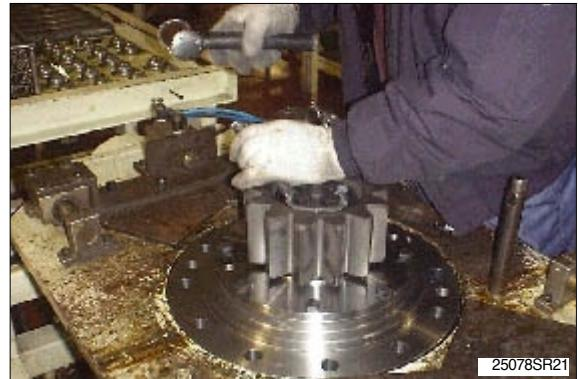
Loosen hex bolt(6) and remove spacer (3) and cover plate by screwing a removal bolt into tap hole on the cover plate(5).
