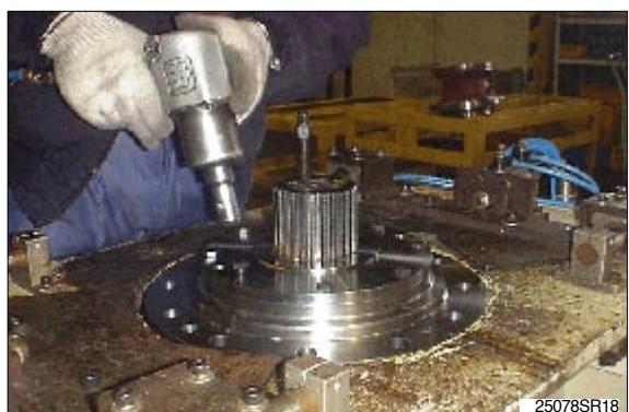
Install pinion gear(25).
