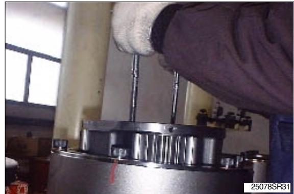
Move out ring gear by the removal groove between ring gear(22) and casing(1) by using removal jig.
