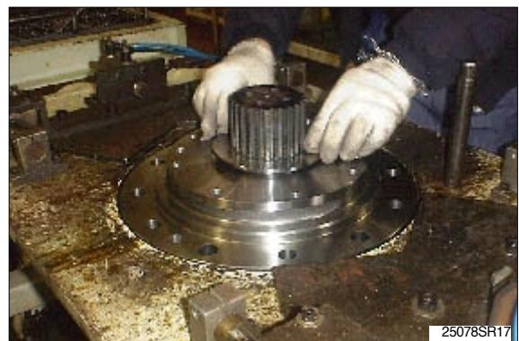
Dismantle drive shaft by using jig
