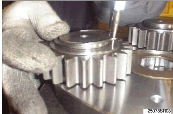
Dismantle needle cage(20) and No.1 side plate(21).
