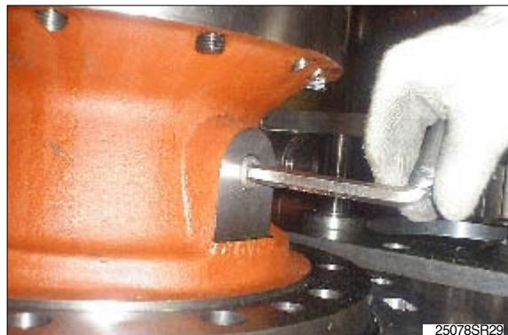
Loosen the socket bolts(24) to separate swing motor from reduction gear.
