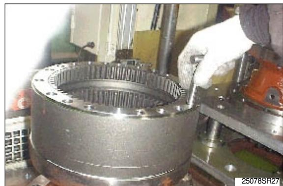
Put it on the working table with drive shaft up.
