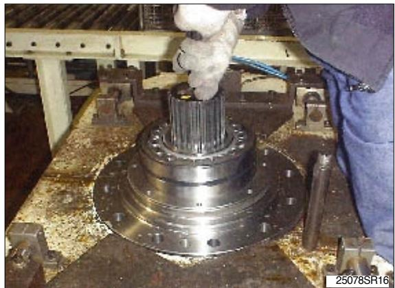
Assemble cover plate(5) and thereafter spacer(3).
