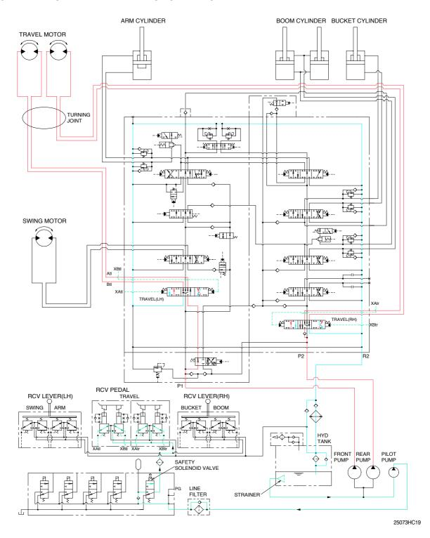
When the right and left travel levers are manually placed to the forward or reverse position, the oil flows from pilot pump through the pilot valve to travel sections of the main control valve.
