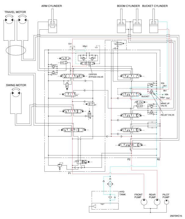
When the RH control lever is manually placed in the bucket roll in position. Then the oil flows from pilot pump through the pilot valve to bucket section of the main control valve. Here the spool position is moved to bucket roll in position.
