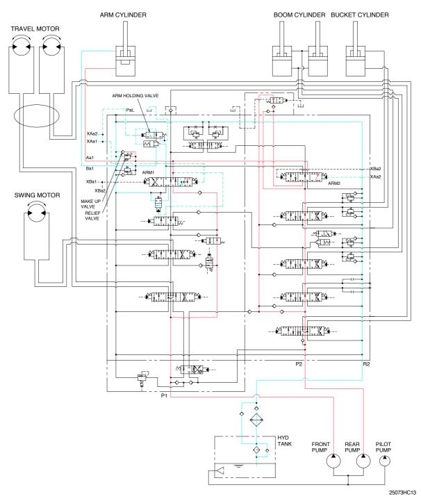
When the LH control lever is pulled back, the arm spools in the main control valve are moved to the roll in position by the pilot oil pressure from the remote control valve.
