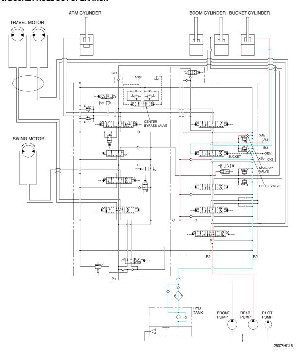
When the RH control lever is manually placed in the bucket roll out position. Then the oil flows from pilot pump through the pilot valve to bucket section of the main control valve. Here the spool position is moved to bucket roll out position.
