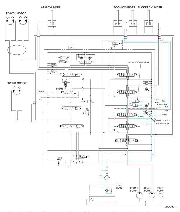
When the RH control lever is pushed forward, the boom spools in the main control valve are moved to the down position by the pilot oil pressure from the remote control valve.
