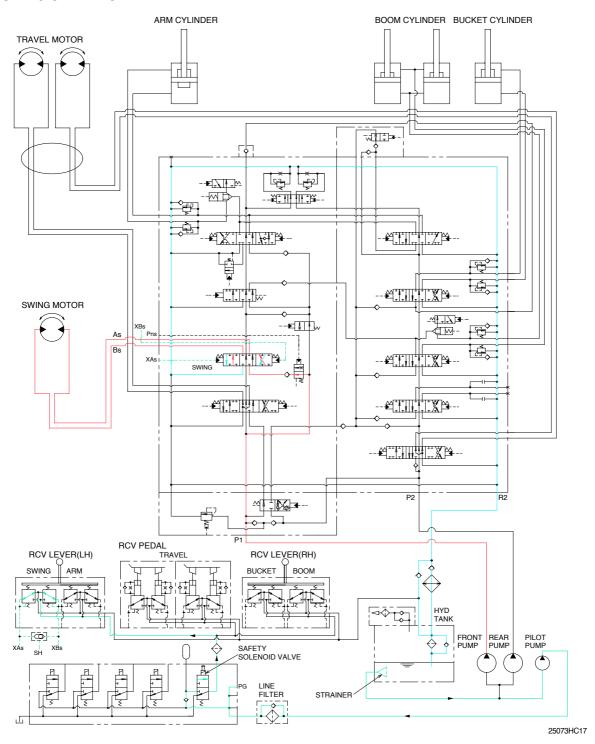
When the LH control lever is manually placed in the left(Right) swing position. Then the oil flows from front pump through the swing section of the main control valve to swing motor to left(Right) swing the superstructure. The return oil flows from swing motor through the swing section of the main control valve returned to the tank.
