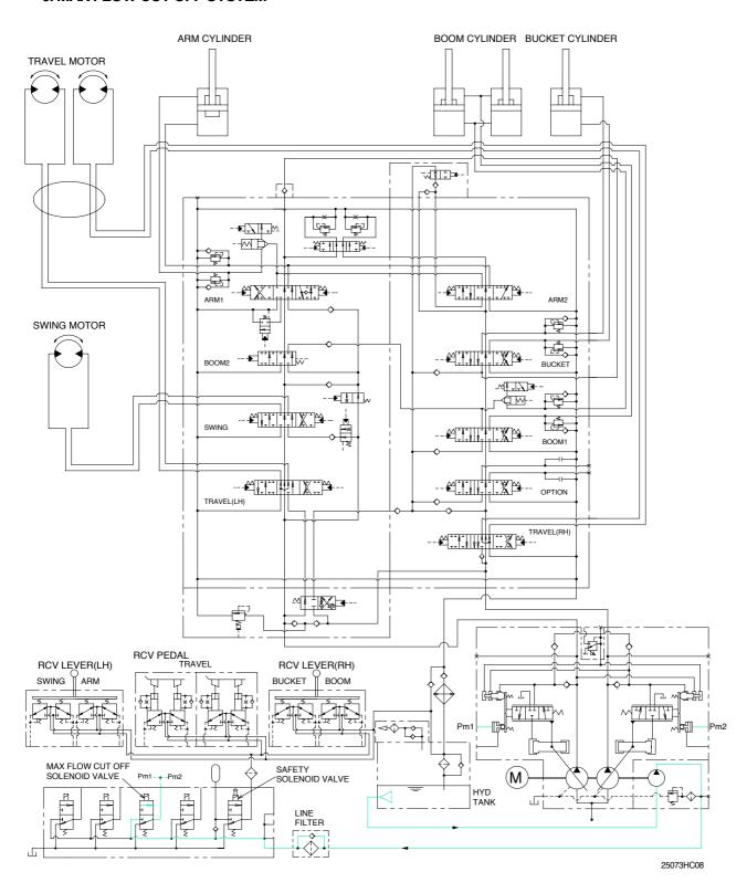
When the breaker operation mode is selected on the cluster, max flow cut off solenoid valve actuates automatically. Thus pilot pressure(Pm1,Pm2) is sent to the regulator and pump discharge volume is decreased.
