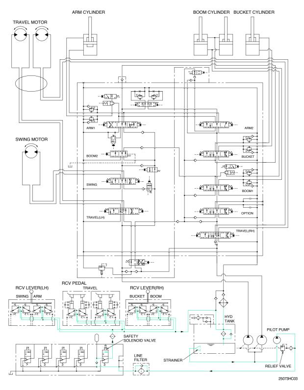
When the travel speed solenoid valve was placed in the Hi position, the pressure oil from pilot pump through line filter flows to port(Pk) of travel speed change over valve, and the control piston is pushed up, thus minimizing the displacement.
