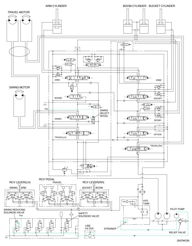
When carrying out the combined operation of swing and boom or arm of the left control valve, the boom or arm speed can be lowered than operating speed of swing. When the heary duty working mode in work mode is selected on the cluster, swing reducing solenoid valve actuates automatically. The oil from pilot pump flows into the solenoid valve through the line filter.
