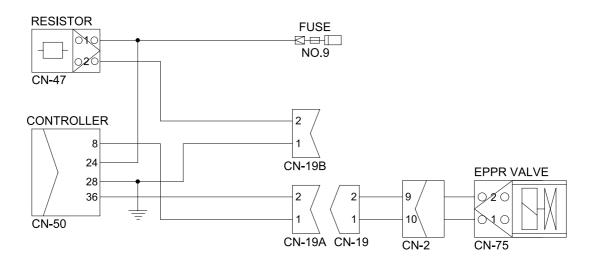
(1) **Test 1 :** Check resistance at connector CN-50(8)-(36).
