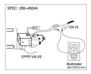
(2) **Test 10**: Check pressure at EPPR valve at S-mode
