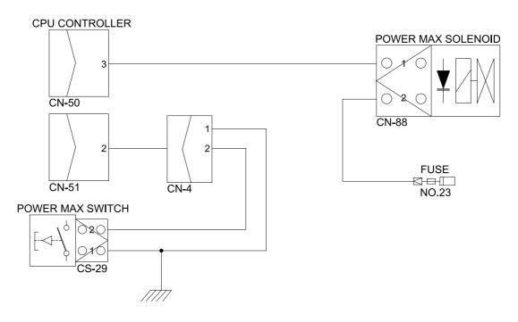
(1) **Test 15:** Check voltage between connector CN-88 - GND.
