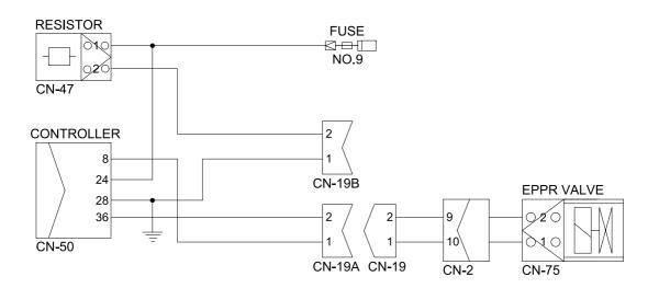
(1) **Test 9 :** Check electric current at EPPR valve at S-mode
