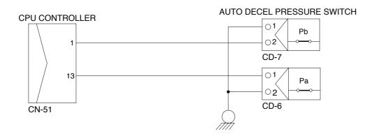
(1) **Test 13**: Check voltage at CN-51(1) and ground.
