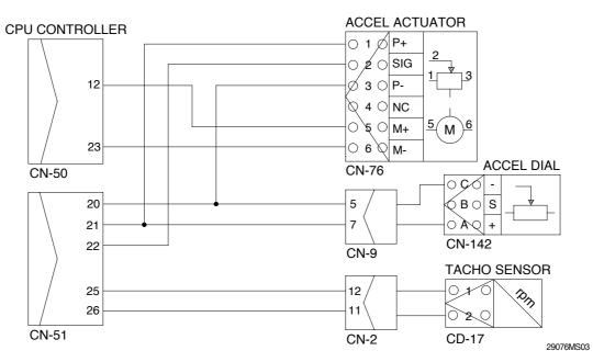
(1) **Test 5**: Check resistance between CN-50 (12)-(23).
