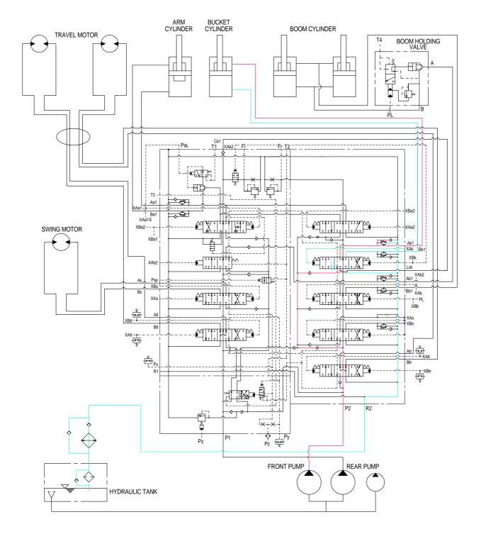
When the right control lever is pushed right, the bucket spool in the main control valve is moved to the roll out position by the pilot oil pressure from the remote control valve.
