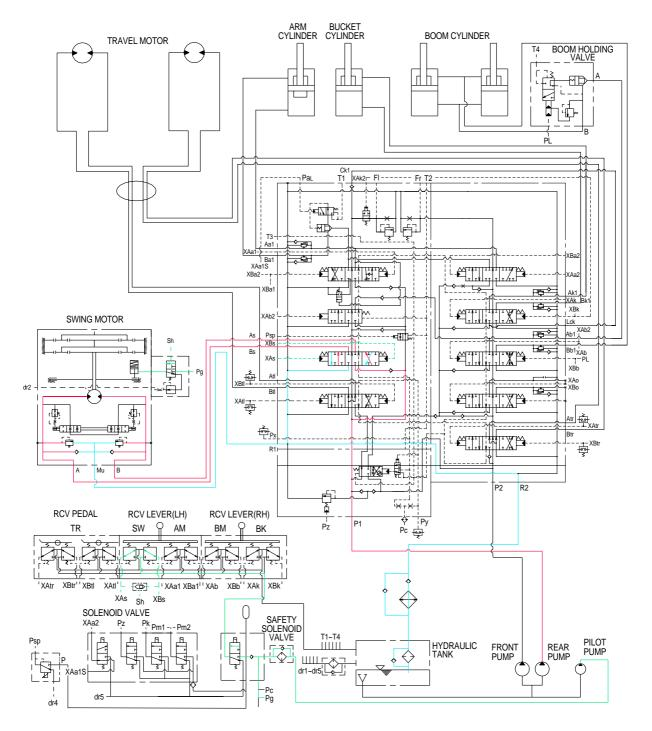
When the left control lever is pushed left or right, the swing spool in the main control valve is moved to the left or right swing position by the pilot oil pressure from the remote control valve.
