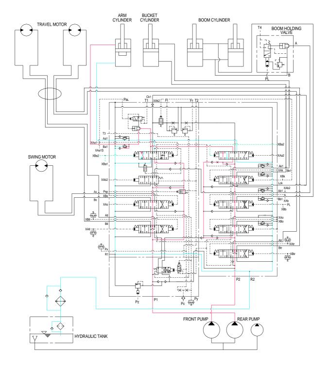
When the left control lever is pushed forward, the arm spool in the main control valve are moved to the roll out position by the pilot oil pressure from the remote control valve.
