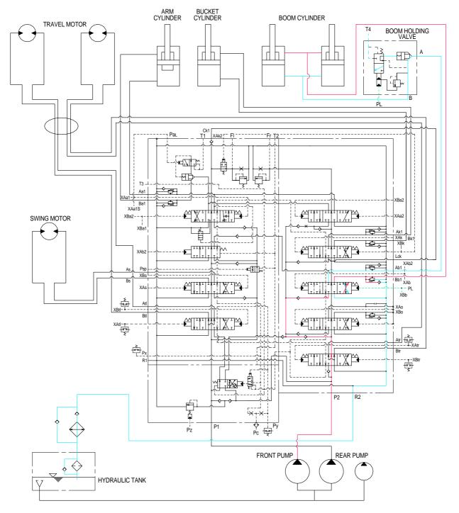
When the right control lever is pushed forward, the boom spools in the main control valve are moved to the lower position by the pilot oil pressure from the remote control valve.
