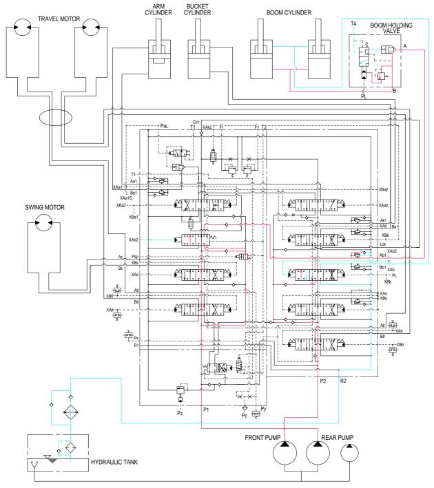
When the right control lever is pulled back, the boom spools in the main control valve are moved to the raise position by the pilot oil pressure from the remote control valve.
