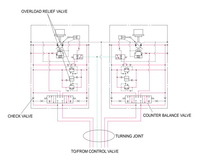
Brake valves are provided on travel motors to offer the following functions.
