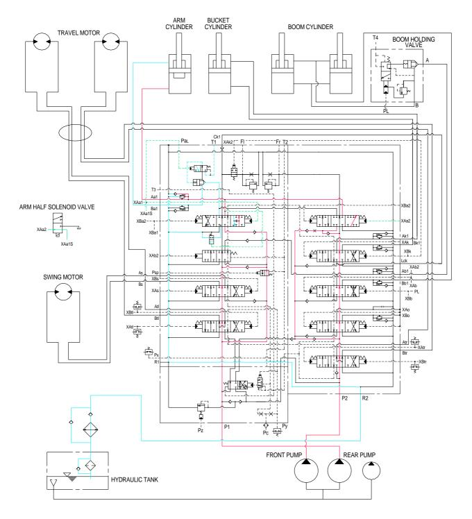
When the left control lever is pulled back the arm spools in the main control valve are moved the to roll in position by the pilot oil pressure from the remote control valve.
