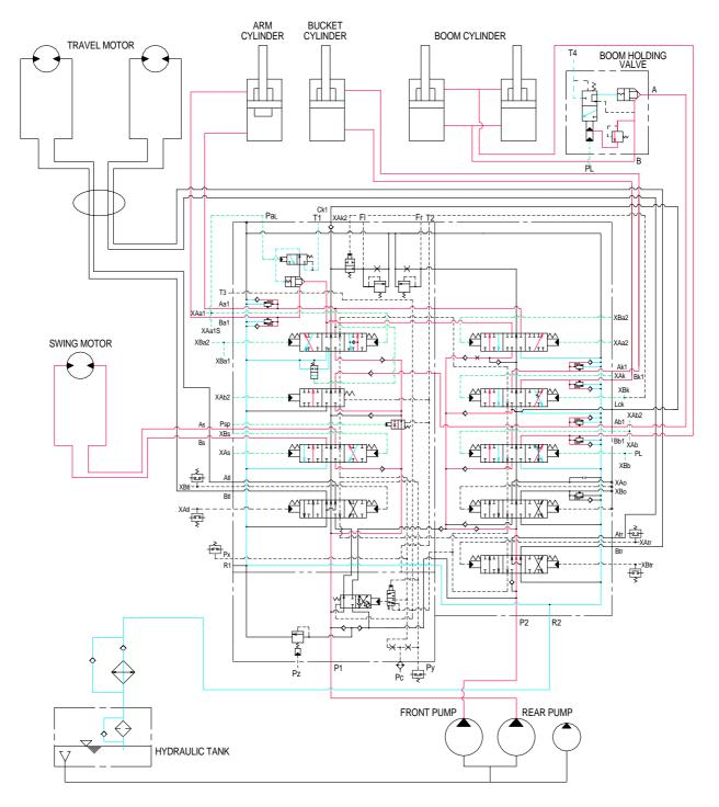
When the swing, boom, arm and bucket functions are operated, simultaneously each spool in the main control valve is moved to the functional position by the pilot oil pressure from the remote control valve.
