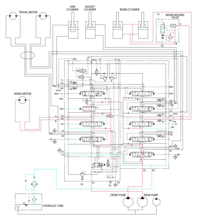
When the swing and boom functions are operated, simultaneously the swing spool and boom spools in the main control valve are moved to the functional position by the pilot oil pressure from the remote control valve.
