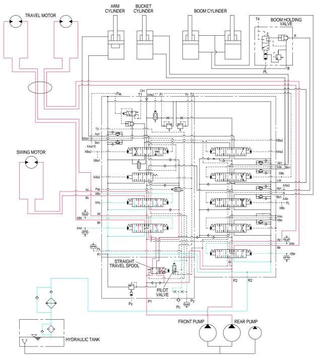
When the swing and travel functions are operated, simultaneously the swing spool and travel spools in the main control valve are moved to the functional position by the pilot oil pressure from the remote control valve and the spool of pilot valve for straight travel is pushed to the downward by the pilot oil pressure from the pilot pump.
