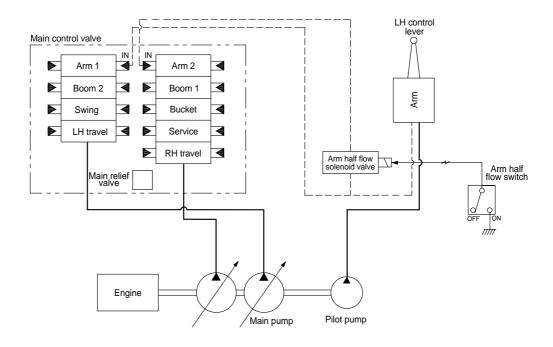
When arm half flow switch is turned ON, the arm half flow solenoid valve is switched to ON and it cancels the junction of the oil flow from two pumps.
