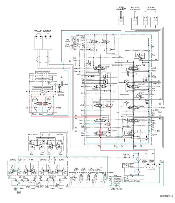
When the left control lever is pushed left or right, the swing spool in the main control valve is moved
