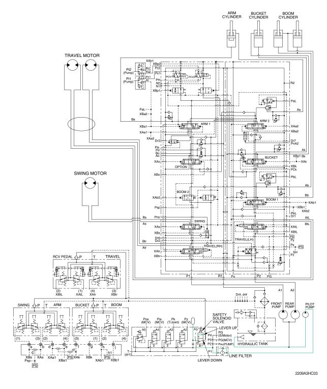
When the lever of the safety solenoid valve is moved upward, oil flows into the remote control valve through solenoid valve and line filter.
