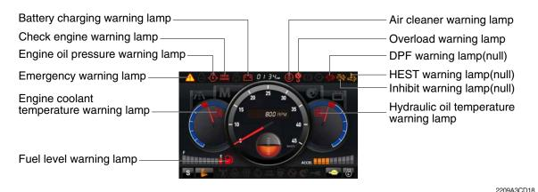
Each warning lamp on the top of the LCD pops up on the center of LCD and the buzzer sounds when the each warning is happened. The pop-up warning lamp moves to the inal position and blinks when the select switch is pushed. And the buzzer stops. Refer to page 5-56 for the select switch.
