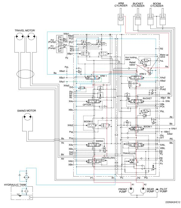
When the left control lever is pushed forward, the arm spools in the main control valve are moved to the roll out position by the pilot oil pressure from the remote control valve.
