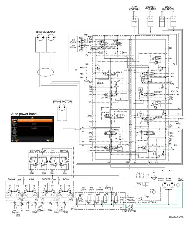
When the power boost switch on the left control lever is pushed ON, the power boost solenoid valve is actuated, the discharged oil from the pilot pump flows into **Pz** port of the main relief valve of main control valve; then the setting pressure of the main relief valve is raised from 350 kgf/cm² to 380 kgf/cm² for increasing the digging power.
