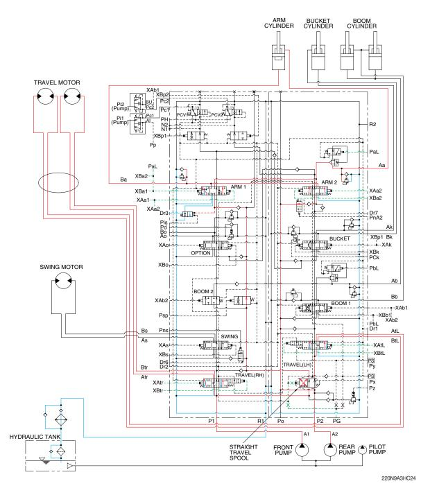
When the arm and travel functions are operated, simultaneously the arm spools and travel spools in the main control valve are moved to the functional position by the pilot oil pressure from the remote control valve and the straight travel spool is pushed to the right by the oil pressure from pilot pump. The oil from the front pump flows into the travel motors through the RH travel spool of the left control
