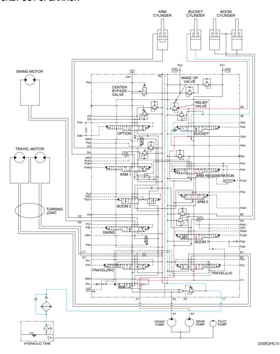
When the RH control lever is manually placed in the bucket roll out position. Then the oil flows from pilot pump through the pilot valve to bucket section of the main control valve. Here the spool position is moved to bucket roll out position.
