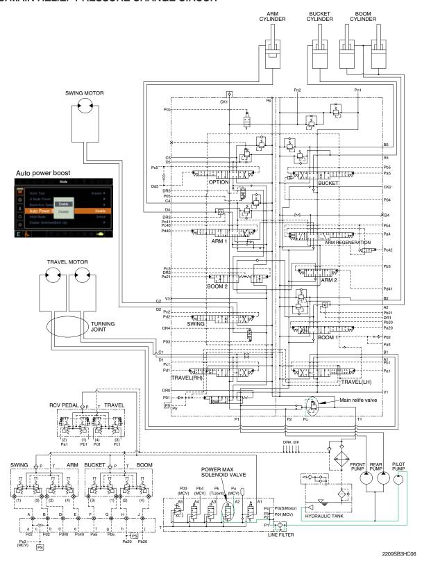
When the power max switch on the left control lever is pushed ON, the power max solenoid valve is actuated, the discharged oil from the pilot pump into Pu port of the main relief valve of main control valve; Then the setting pressure of the main control valve is raises from 350 kgf/cm² to 380 kgf/cm² for increasing the digging power. And even when press continuously, it is canceled after 8 seconds.
