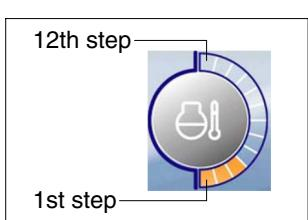
① This gauge indicates the temperature of coolant in 12 step gauge.
