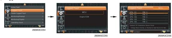
· The logged faults of the MCU or engine ECM can be checked by this menu.
