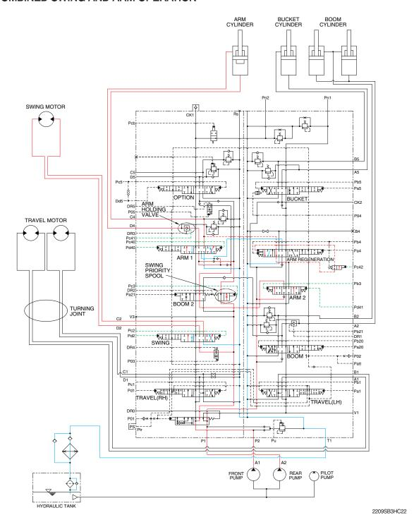
When the swing and arm functions are operated, simultaneously the swing spool and arm spools in the main control valve are moved to the functional position by the pilot oil pressure from the remote control valve.
