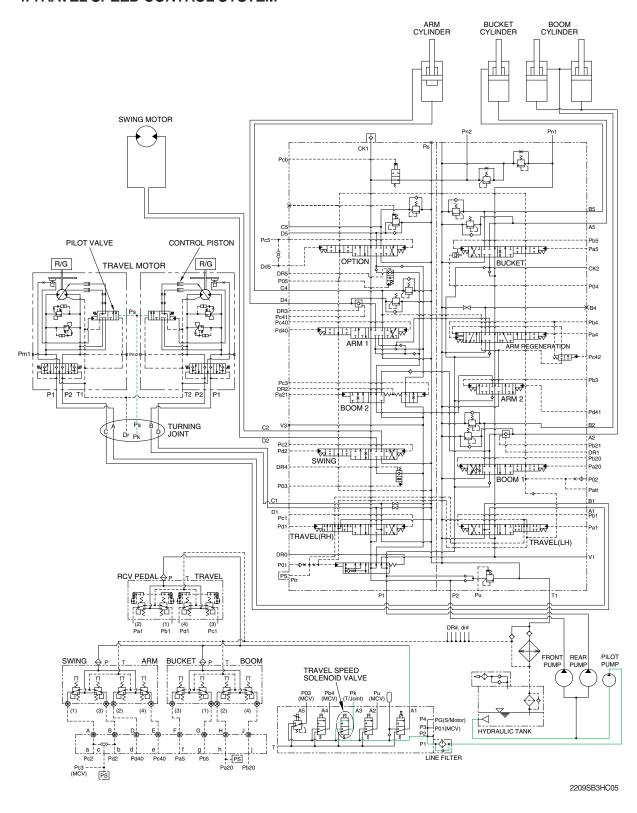
When the travel speed solenoid valve was placed in the Hi position, the pressure oil from pilot pump through line filter flows to port **Ps** of travel speed change over valve, and the control piston is pushed up, thus minimizing the displacement.
