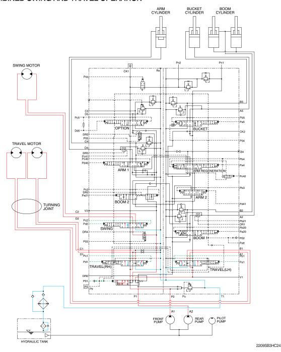
When the swing and travel functions are operated, simultaneously the swing spool and travel spools in the main control valve are moved to the functional position by the pilot oil pressure from the remote control valve. At the same time, the straight travel spool is pushed to the right by the pilot oil pressure from the pilot pump.
