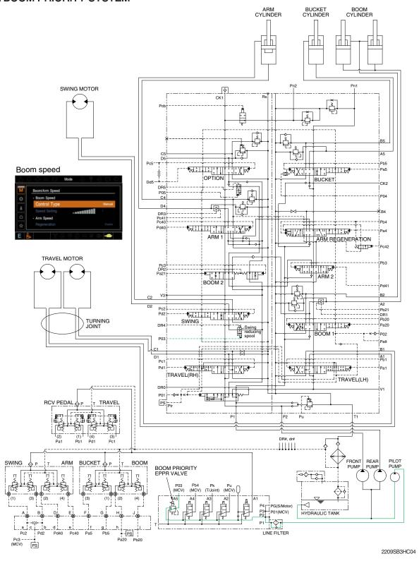
When carrying out the combined operation of swing and boom up, the boom up operating speed is slower than normal operation.
