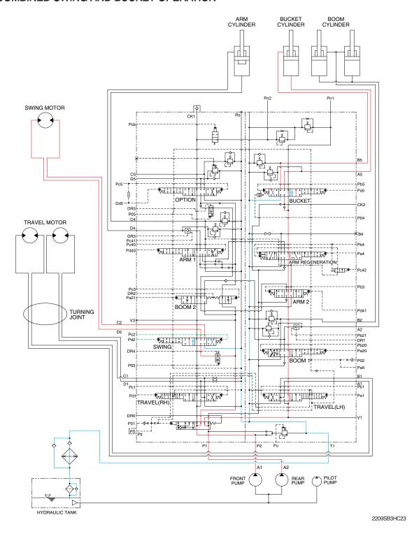
When the swing and bucket functions are operated, the swing and bucket spools changed. The oil flows from the A2 pump through the bucket section of the main control valve to the bucket cylinder and the bucket functions. The oil flows from A1 pump through swing section of the main control valve to the swing motor and swing the superstructure.
