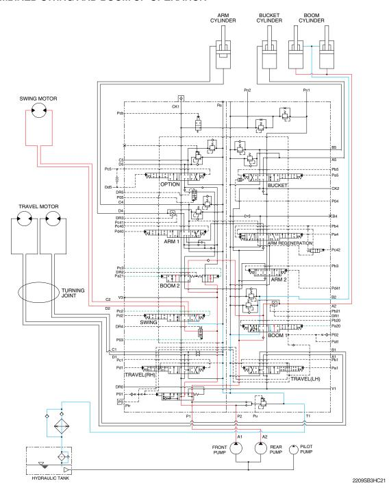
When the swing and boom up functions are operated, simultaneously the swing spool and boom spools changed. The oil flows from the A2 pump through boom1 section of the main control valve to boom cylinders and the boom functions.
