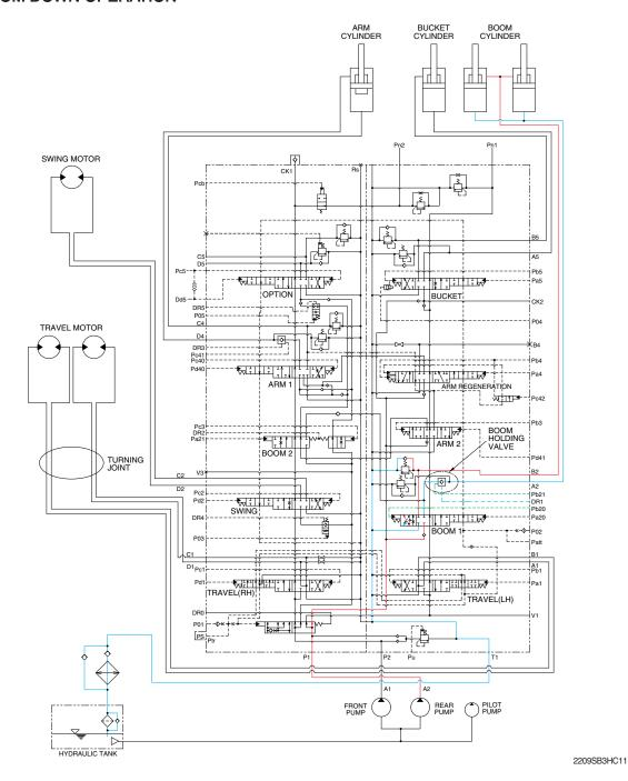
When the RH control lever is pushed forward, the boom spools in the main control valve are moved to the down position by the pilot oil pressure from the remote control valve.
