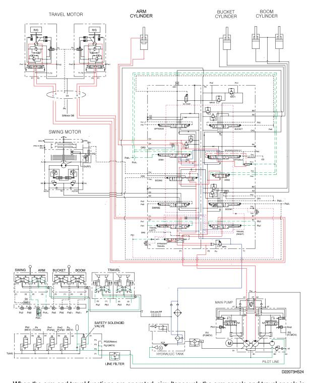
When the arm and travel functions are operated, simultaneously the arm spools and travel spools in the main control valve are moved to the functional position by the pilot oil pressure from the remote control valve and the straight travel spool is pushed to the left by the oil pressure from pilot pump.
