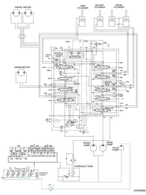
When carrying out the combined operation of swing and boom or arm, the boom or arm operating speed is lowered then normal operation.
