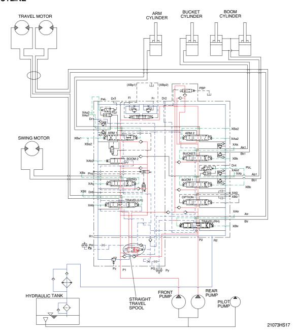
The oil from the front and rear pump flows through the neutral oil passage, bypass oil passage and confluence oil passage in the main control valve. Then the oil goes to each actuator and operates them. Check valves and orifices are located on these oil passage in the main control valve. These control the oil from the main pumps so as to correspond to the operation of each actuator and smooth the combined operation.
