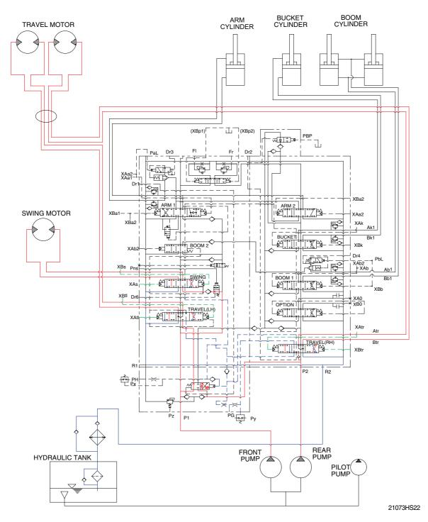
When the swing and travel functions are operated, simultaneously the swing spool and travel spools in the main control valve are moved to the functional position by the pilot oil pressure from the remote control valve and straight travel spool is pushed to the left by the pilot oil pressure from the pilot pump.
