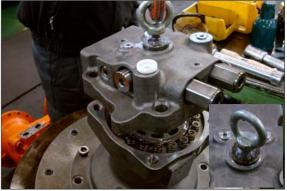
Assemble level gauge(44) into body(1).
