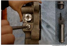
4 Assemble relief valve assy(33) 2set into rear cover(21) with a torque wrench. (Bilateral symmetry assembling)
