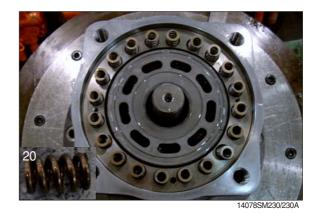
(3) Assemble the sub of rear cover assy sub
