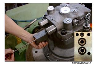
② Disassemble level gauge(44) from body (1).
