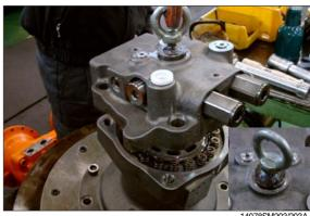
4 Using a jig, disassemble break piston(17) from body(1).
