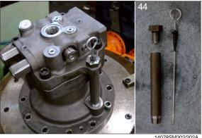
① Assemble time delay valve assy(35) into rear cover(21) with a wrench bolt(36).
