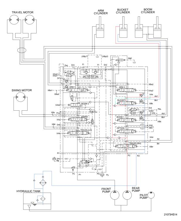
When the right control lever is pushed right, the bucket spool in the main control valve is moved to the roll out position by the pilot oil pressure from the remote control valve.
