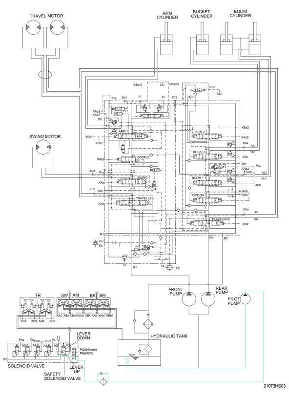
When the lever of the safety solenoid valve is moved downward, oil flows into the remote control valve through solenoid valve and line filter.
