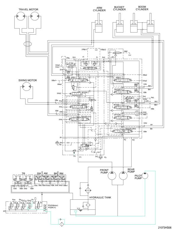
When the power boost switch on the left control lever is pushed ON, the power boost solenoid valve is actuated, the discharged oil from the pilot pump flows into Pz port of the main relief valve of main control valve; then the setting pressure of the main relief valve is raised from 330kgf/cm<sup>2</sup> to 360kgf/cm<sup>2</sup> for increasing the digging power. And even when pressed continuously, it is canceled after 8 seconds.
