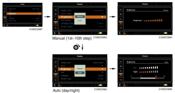
If "Auto" is chosen, brightness for day and night can be differently set up. Also by using the bar in lower side, users can define which time interval belongs to day and night.
