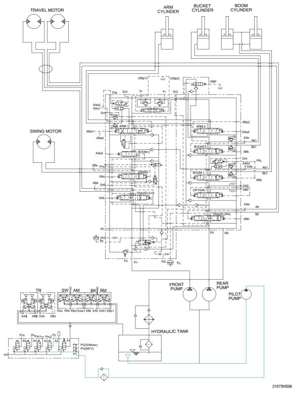
When the power boost switch on the left control lever is pushed ON, the power boost solenoid valve is actuated, the discharged oil from the pilot pump flows into Pz port of the main relief valve of main control valve; then the setting pressure of the main relief valve is raised from 330kgf/cm² to 360kgf/cm² for increasing the digging power. And even when pressed continuously, it is canceled after 8 seconds.
