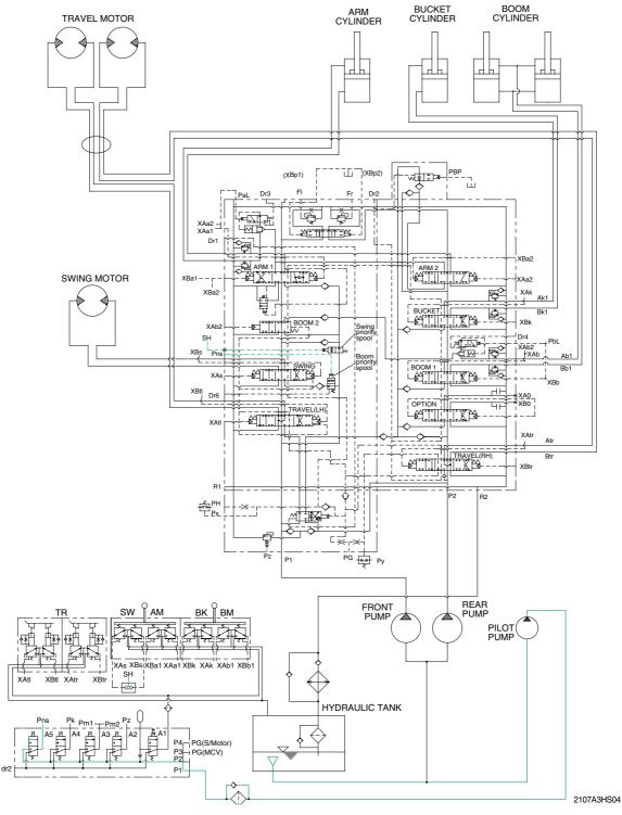
When carrying out the combined operation of swing and boom or arm, the boom or arm operating speed is lowered then normal operation. The oil pressure from the swing shuttle port(SH) change the swing priority spool and decrease the oil flow rate to the next section.
