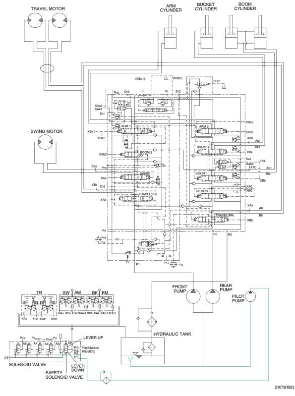
When the lever of the safety solenoid valve is moved upward, oil flows into the remote control valve through solenoid valve and line filter.
