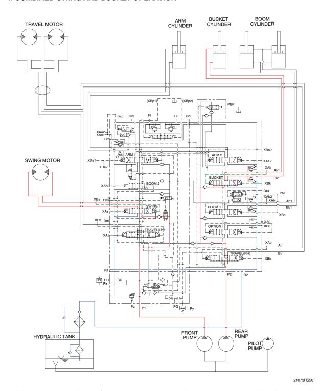
When the swing and bucket functions are operated, simultaneously the swing spool and bucket spool in the main control valve are moved to the functional position by the pilot oil pressure from the remote control valve.
