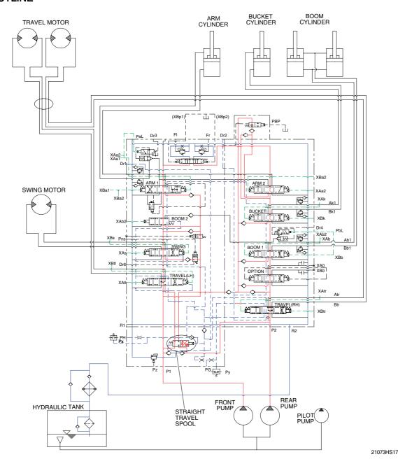
The oil from the front and rear pump flows through the neutral oil passage, bypass oil passage and confluence oil passage in the main control valve. Then the oil goes to each actuator and operates them. Check valves and orifices are located on these oil passage in the main control valve. These control the oil from the main pumps so as to correspond to the operation of each actuator and smooth the combined operation.
