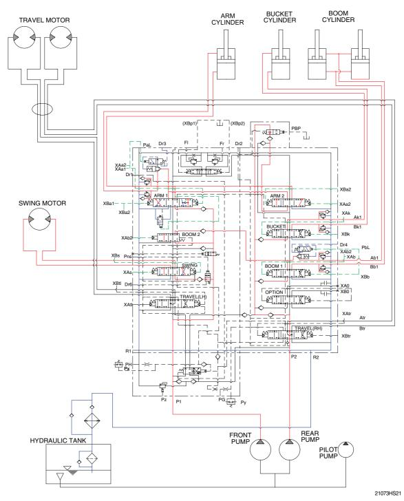
When the swing, boom, arm and bucket functions are operated, simultaneously each spool in the main control valve is moved to the functional position by the pilot oil pressure from the remote control valve.
