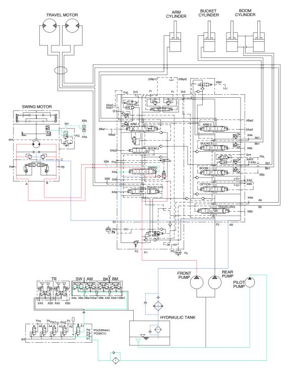
When the left control lever is pushed left or right, the swing spool in the main control valve is moved to the left or right swing position by the pilot oil pressure from the remote control valve.
