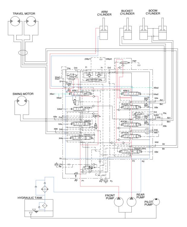
When the left control lever is pushed forward, the arm spool in the main control valve are moved to the roll out position by the pilot oil pressure from the remote control valve.
