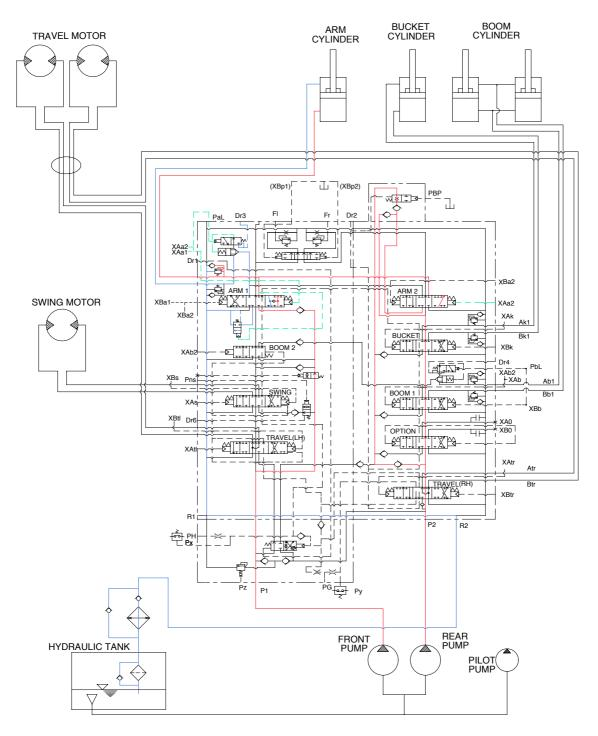
When the left control lever is pulled back, the arm spools in the main control valve are moved the to roll in position by the pilot oil pressure from the remote control valve.
