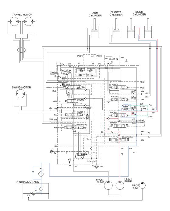
When the right control lever is pushed forward, the boom spools in the main control valve are moved to the down position by the pilot oil pressure from the remote control valve.
