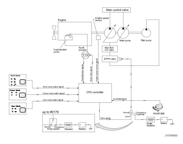
Mode selection system(Micro computer based electro-hydraulic pump and engine mutual control system) optimizes the engine and pump performance.
