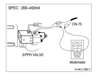
(2) **Test 4 :** Check pressure at EPPR valve at S-mode
