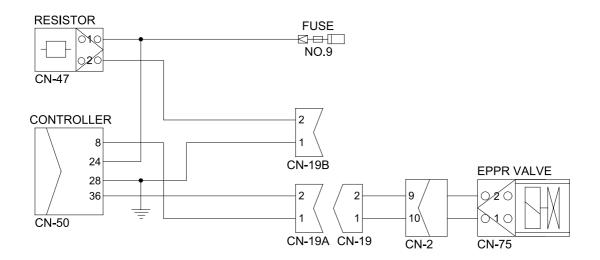
(1) **Test 9 :** Check electric current at EPPR valve at S-mode
