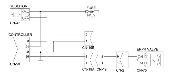
(1) **Test 3**: Check electric current at EPPR valve at S-mode
