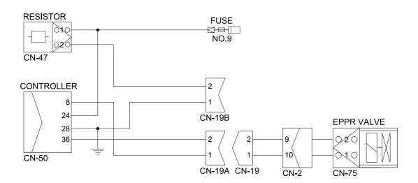
(1) **Test 1 :** Check resistance at connector CN-50(8)-(36).
