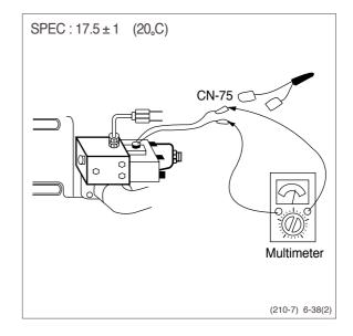
(3) **Test 3 :** Check electric current at EPPR valve. Install multimeter as figure.
