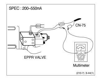
(2) **Test 10**: Check pressure at EPPR valve at S-mode
