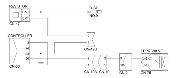
(1) **Test 2 :** Check resistance at connector CN-75.
