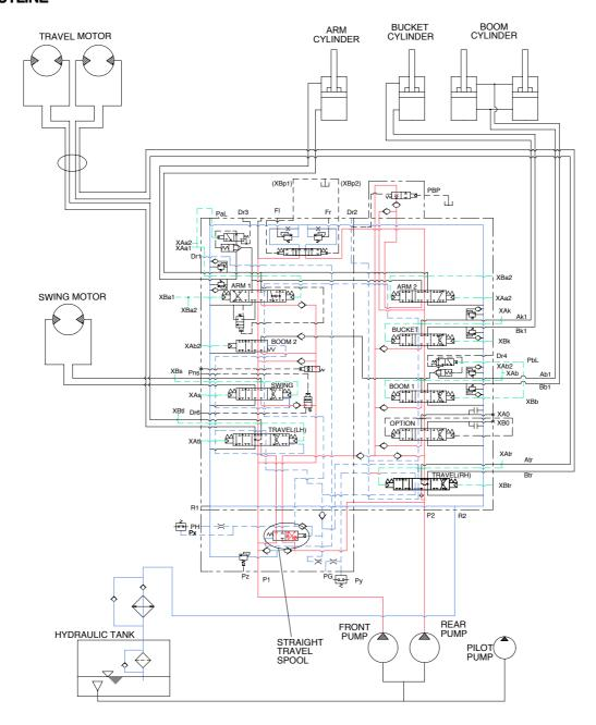
The oil from the front and rear pump flows through the neutral oil passage, bypass oil passage and confluence oil passage in the main control valve. Then the oil goes to each actuator and operates them. Check valves and orifices are located on these oil passage in the main control valve. These control the oil from the main pumps so as to correspond to the operation of each actuator and smooth the combined operation.
