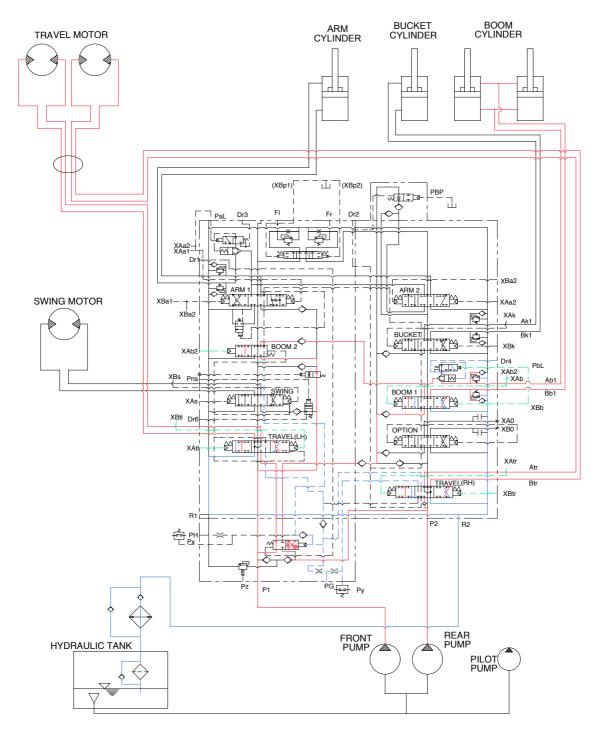
When the boom and travel functions are operated, simultaneously the boom spools and travel spools in the main control valve are moved to the functional position by the pilot oil pressure from the remote control valve and the straight travel spool is pushed to the left by the oil pressure from pilot pump.
