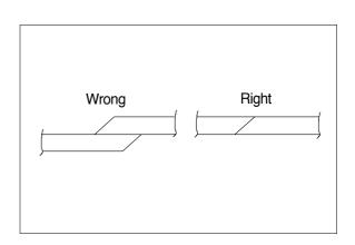
Rod seal(6) has its own fitting direction. Therefore, confirm it before fitting them. Fitting rod seal(6) upside down may damage its lip. Therefore check the correct direction that is shown in fig.
