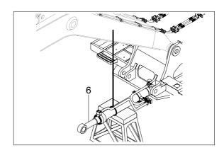
Disconnect boom cylinder hoses(7) and put plugs on cylinder pipe.
