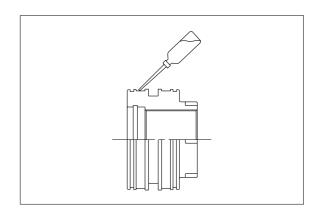
Fit piston seal(17) to piston.
