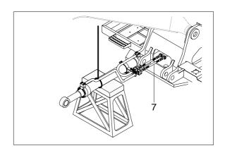
Remove bolt(9) and pull out pin(8). Remove boom cylinder assembly(6).
