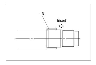
Fit piston assembly to rod assembly.
