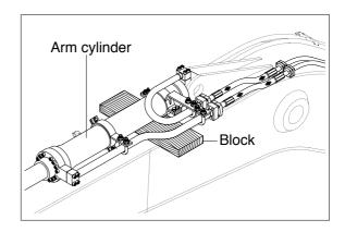
Remove bolt(2) and pull out pin(1). Tie the rod with wire to prevent it from coming out.
