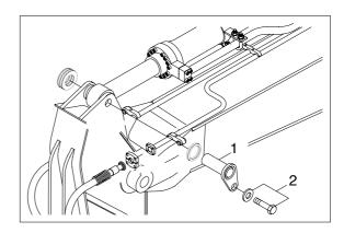
Disconnect arm cylinder hoses(4) and put plugs on cylinder pipe.
