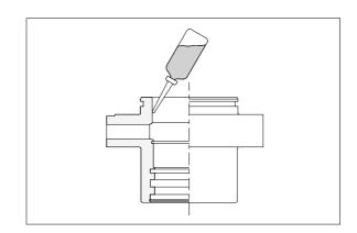
Coat dust wiper(9) with grease and fit dust wiper(9) to the bottom of the hole of dust seal.
