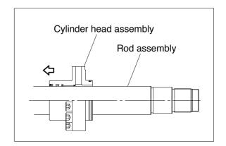
Insert cushion ring(13) to rod assembly. Note that cushion ring(13) has a direction in which it should be fitted.
