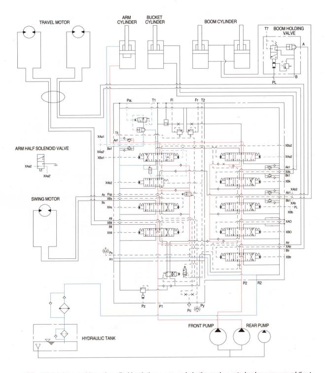
When the left control lever is pulled back the arm spools in the main control valve are moved the to roll in position by the pilot oil pressure from the remote control valve.
