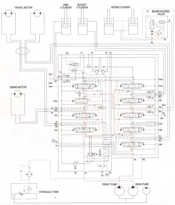
When the right control lever is pulled back, the boom spools in the main control valve are moved to the raise position by the pilot oil pressure from the remote control valve.
