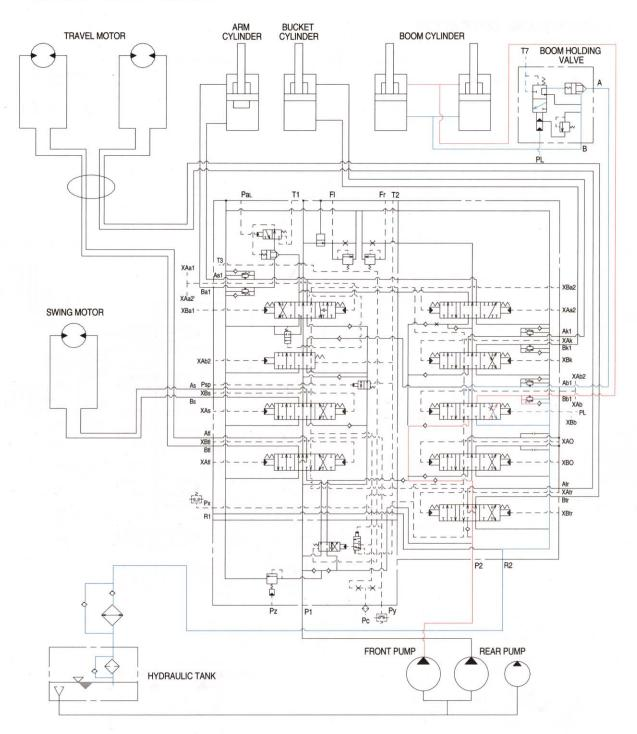
When the right control lever is pushed forward, the boom spools in the main control valve are moved to the lower position by the pilot oil pressure from the remote control valve.
