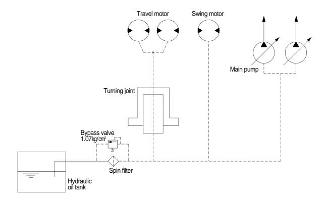
Besides internal leaks from the motors and main pump, the oil for lubrication circulates. These oil have to be fed to the hydraulic tank passing through spin filter.
