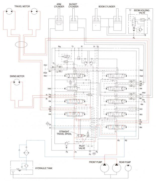
When the swing and travel functions are operated, simultaneously the swing spool and travel spools in the main control valve are moved to the functional position by the pilot oil pressure from the remote control valve and the spool of pilot valve for straight travel is pushed to the downward by the pilot oil pressure from the pilot pump.
