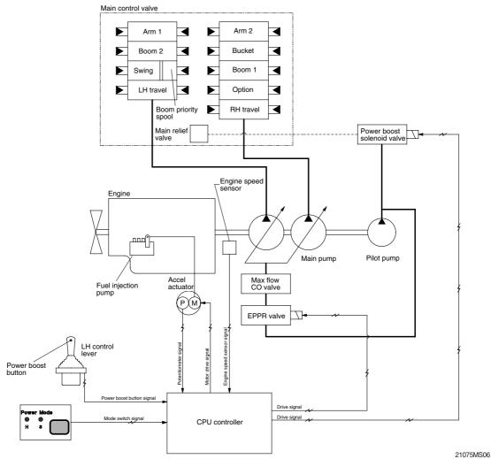
on the left control lever knob is pushed ON, the maximum diagin
