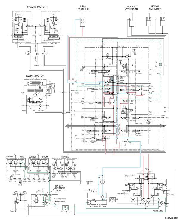
When the left control lever is pulled back, the arm spools in the main control valve are moved to the roll in position by the pilot oil pressure from the remote control valve.
