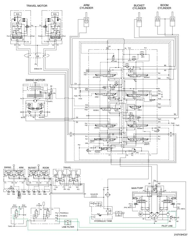
When the breaker operation mode is selected on the cluster, max flow cut off solenoid valve actuates automatically.
