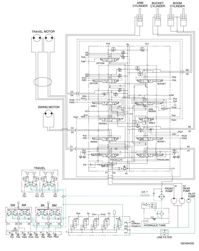
The pilot pump receive oil from the hydraulic tank. The discharged oil from the pilot pump flows to the safety solenoid valve through the line filter. The oil is filtered by the line filter. The pilot relief valve is provided in the pilot pump for limiting the pilot circuit pressure.
