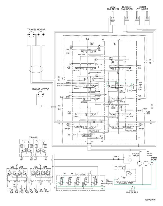
Then the heavy duty mode switch on the cluster is pushed ON, the arm regeneration solenoid valve is deactivated and the arm regeneration spool is returned to neutral position.
