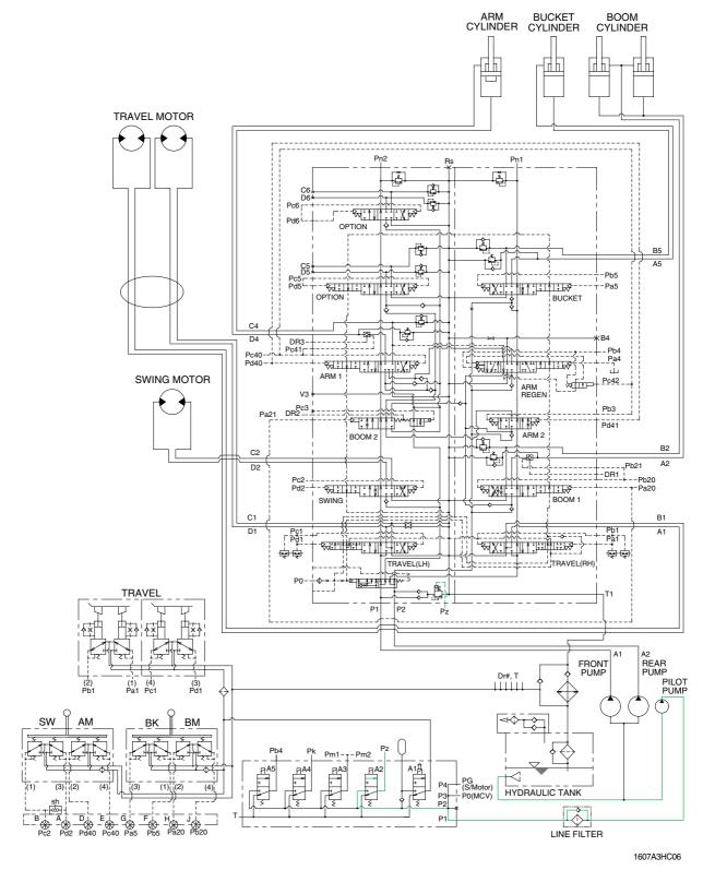
When the power boost switch on the left control lever is pushed ON, the power boost solenoid valve is actuated, the discharged oil from the pilot pump flows into Pz port of the main relief valve of main control valve; then the setting pressure of the main relief valve is raised from 330kgf/cm² to 360kgf/cm² for increasing the digging power. And even when pressed continuously, it is canceled after 8 seconds.
