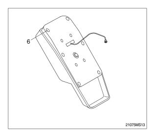
Install the new ROM.(Be careful of direction and assemble the cluster in the reverse order to removal).
