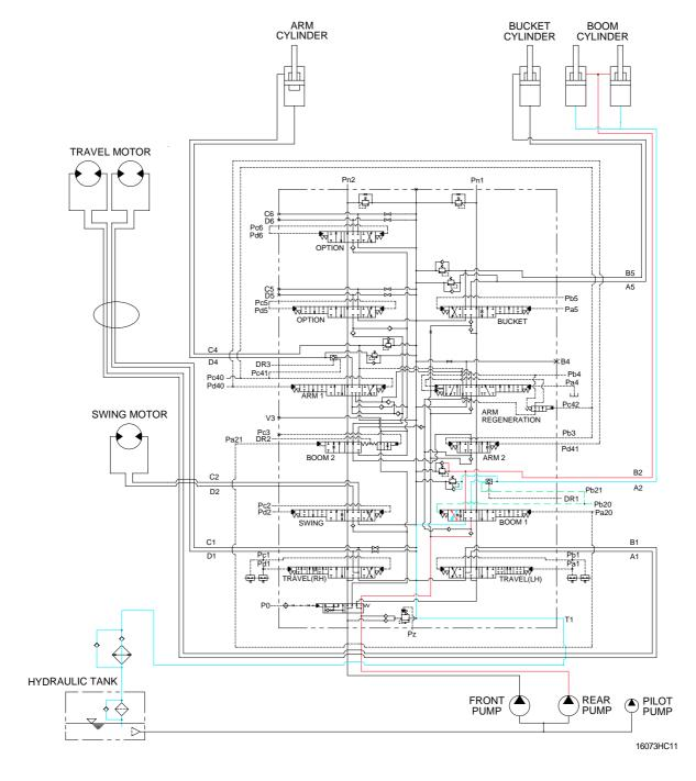
When the right control lever is pushed forward, the boom spools in the main control valve are moved to the down position by the pilot oil pressure from the remote control valve.
