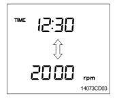
This displays the current time and machine information such as engine rpm, coolant/hydraulic oil temperature, hydraulic oil pressure and also error codes.
