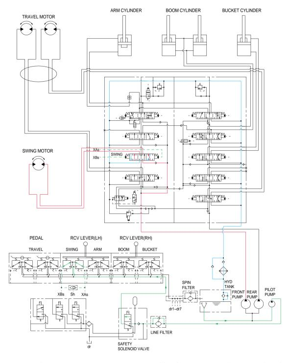
When the left control lever is manually placed in the left(right) swing position. Then the oil flows from front pump through the swing section of the main control valve to swing motor to left(right) swing the superstructure. The return oil flows from swing motor through the swing section of the main control valve returned to the tank.
