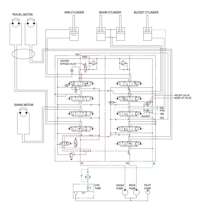
When the right control lever in manually placed in the bucket roll in position. Then the oil flows from pilot through the pilot valve to bucket section of the main control valve. Here the spool position is moved to bucket roll in position.
