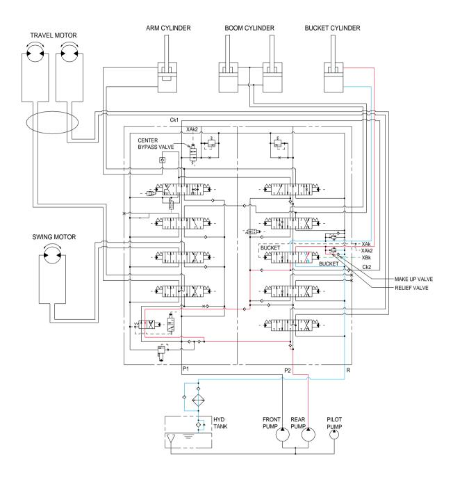
When the right control lever in manually placed in the bucket roll out position. Then the oil flows from pilot pump through the pilot valve to bucket section of the main control valve. Here the spool position is moved to bucket roll out position.
