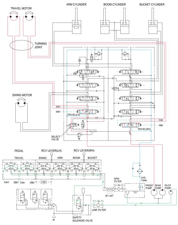
When the right and left travel levers are manually placed to the forward or reverse position. Then the oil flows from pilot pump through the pilot valve to travel sections of travel sections of the main control valve.
