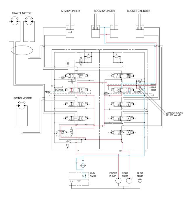
When the right control lever is pulled to boom raise position, the oil flows from pilot pump through the remote control valve to boom sections of the main control valve.
