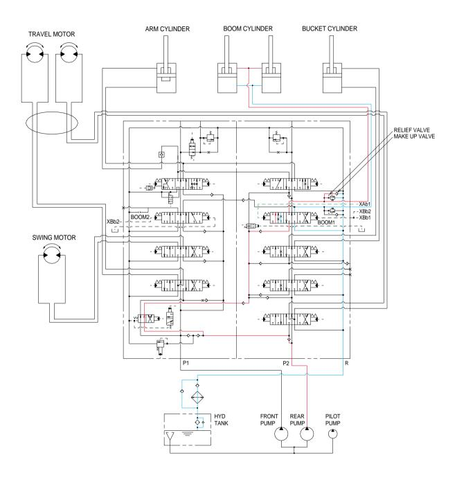
When the right control lever is pushed forward to boom down position, the oil flows from pilot pump through the remote control valve to boom section of the main control valve. Here, the spool positions are move to the boom down position, and the boom down circuit is opened.
