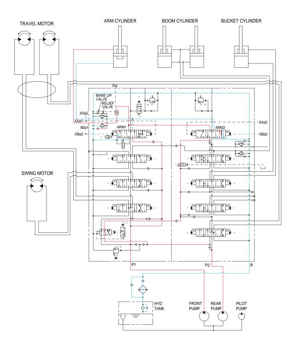
When the left control lever manually is placed in the arm roll out position.
