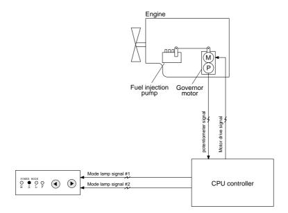
If there is any abnormality in the governor motor system, for instance short or open circuit happens among wire-harness connected to CPU controller, the cluster displays the detected abnormality by glittering 2 mode lamps alternately.
