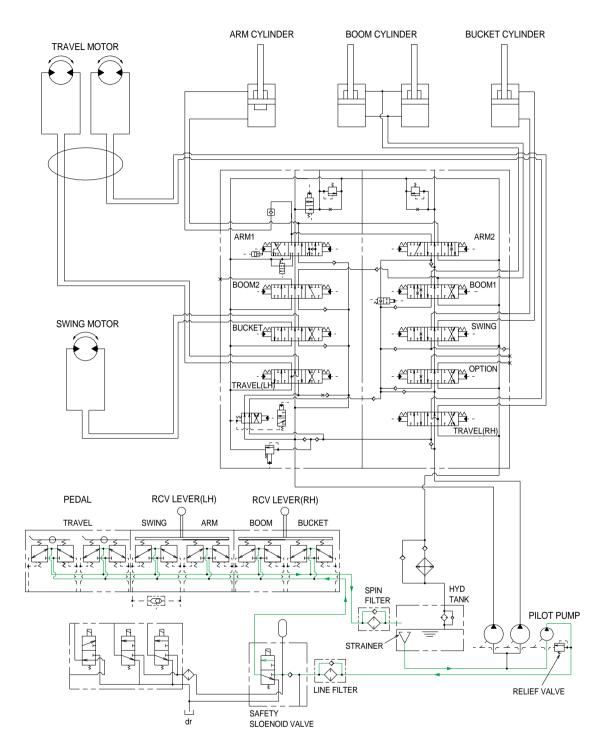
The pilot pump receive oil from the hydraulic tank. The discharged oil from the pilot pump flows to the safely solenoid valve through the line filter. The oil is filtered by the line filter. The pilot relief valve is provided in the pilot pump for limiting the pilot circuit pressure.
