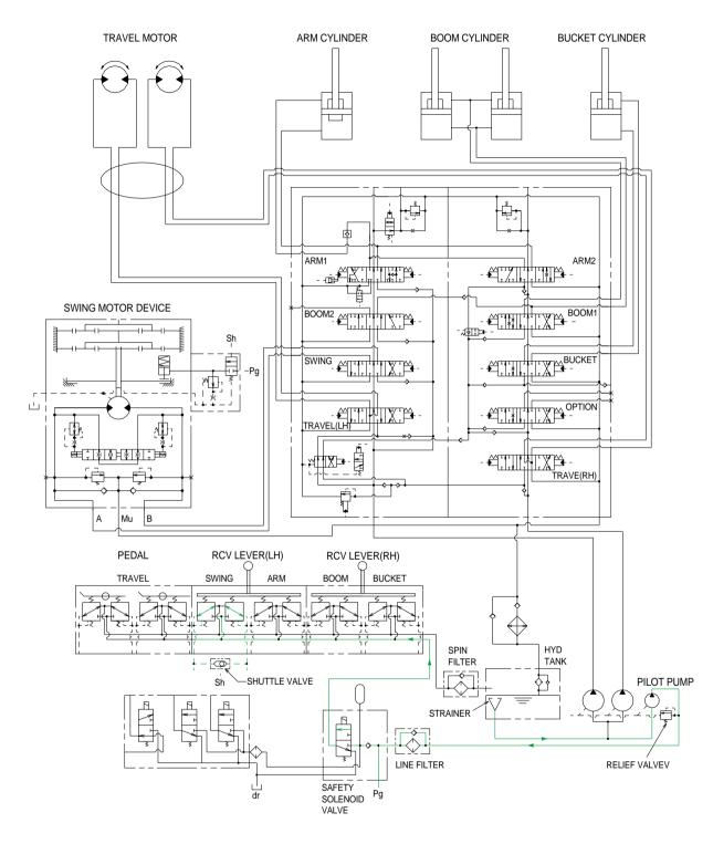
When the swing control lever is operated, the pilot oil flows to Sh port of shuttle valve, this pressure move spool so, discharged oil from pilot pump flows to Pg, port.
