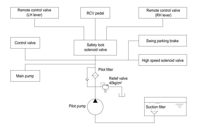
The pilot circuit consists of suction circuit, delivery circuit and return circuit.
