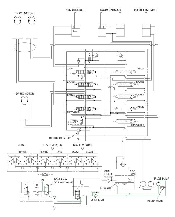
When the power max switch on the left control lever is pushed ON, the power max solenoid valve is actuated, the discharge oil from the pilot pump flows into PZ port of the main relief valve of main control valve ; then the setting pressure of the main control valve is raises from 320kgf/cm<sup>2</sup> to 350kgf/cm<sup>2</sup> for increasing the digging power. And even when pressed continuously, it is canceled after 8 seconds.
