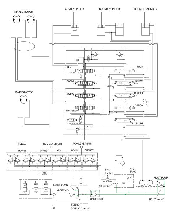
When the lever of the safety solenoid valve moved downward, oil flows into the remote control valve through solenoid valve and line filter.
