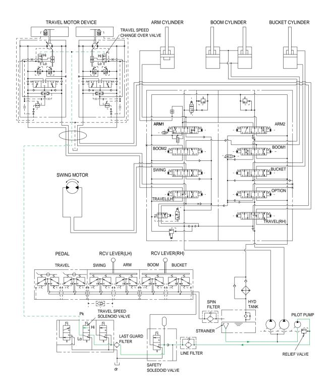
When the travel speed solenoid valve was placed in the Hi position, the pressure oil from pilot pump through last guard filter flows to port(Pk) of travel speed change over valve, and the control piston is pushed up, thus minimizing the displacement.
