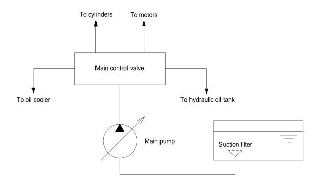
The pumps receive oil from the hydraulic tank through a suction filter. The discharged oil from the pump flows into the control valve and goes out the tank ports.
