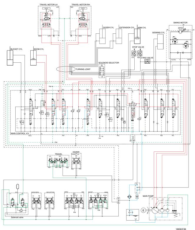
When the boom and travel functions are operated, simultaneously the boom spools and travel spools in the main control valve are moved to the functional position by the pilot oil pressure from the remote control valve.
