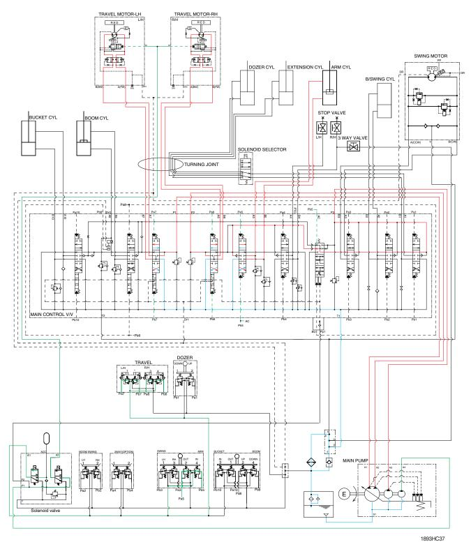
When the arm and travel functions are operated, simultaneously the arm spools and travel spools in the main control valve are moved to the functional position by the pilot oil pressure from the remote control valve.
