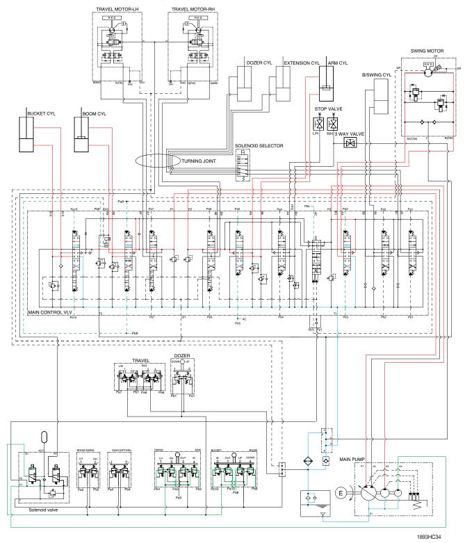
When the swing, boom, arm and bucket functions are operated, simultaneously each spool in the main control valve is moved to the functional position by the pilot oil pressure from the remote control valve.
