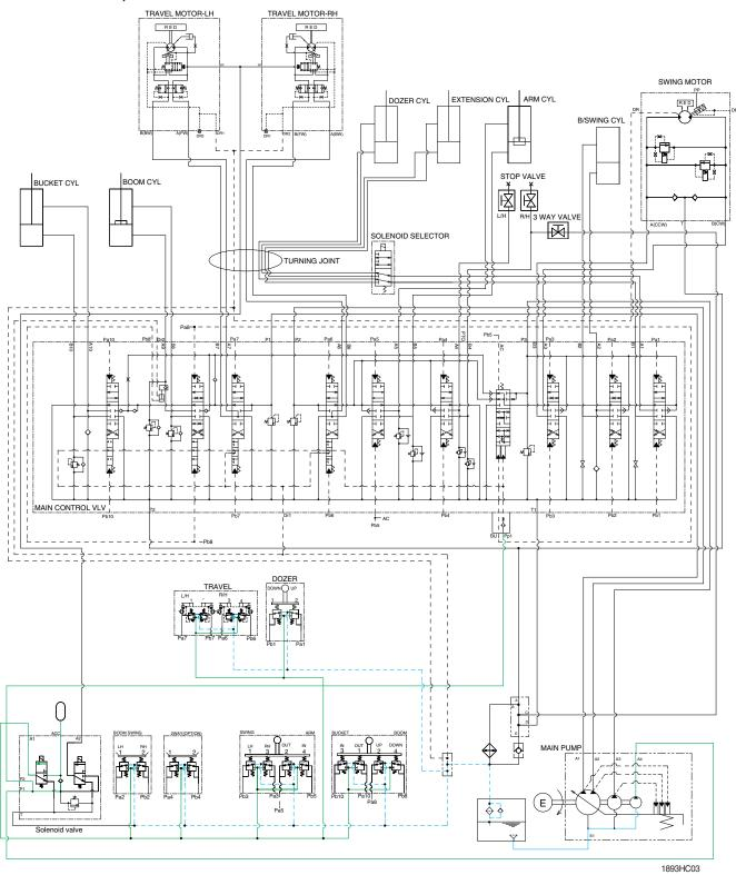
The pilot pump receive oil from the hydraulic tank. The discharged oil from the pilot pump flows to the safety solenoid valve. The pilot relief valve is provided in the solenoid valve for limiting the pilot circuit pressure.
