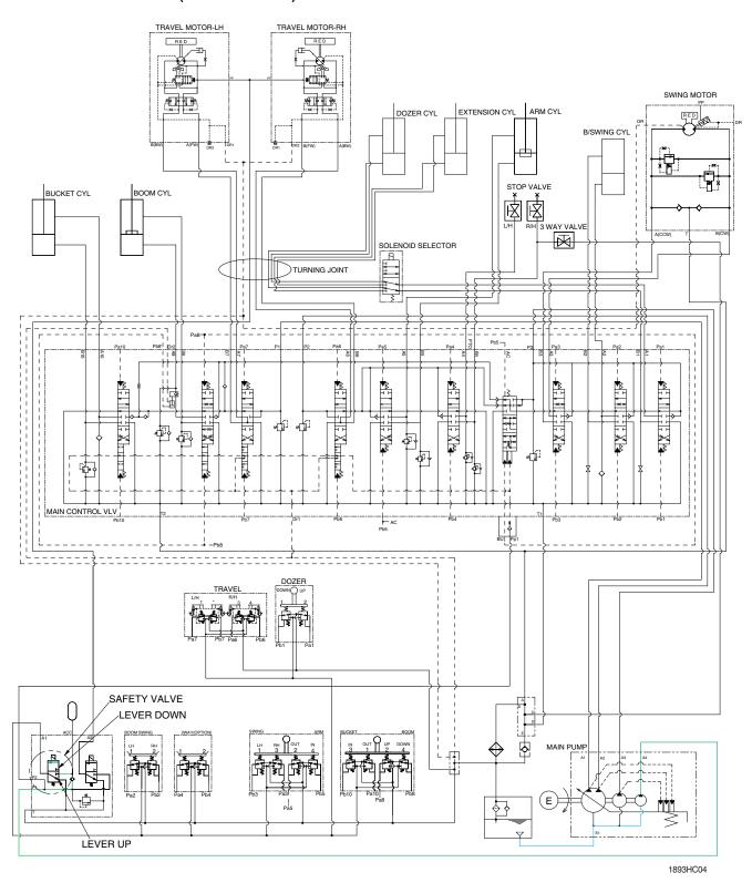
When the lever of the safety solenoid valve is moved downward, oil flows into the remote control valve through solenoid valve.
