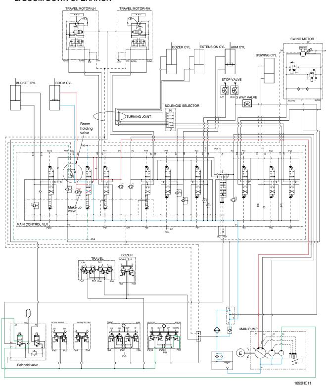
When the right control lever is pushed forward, the boom spools in the main control valve are moved to the down position by the pilot oil pressure from the remote control valve. Since Pb8 port is connected Pb8' port through the piping, boom holding valve is also released.
