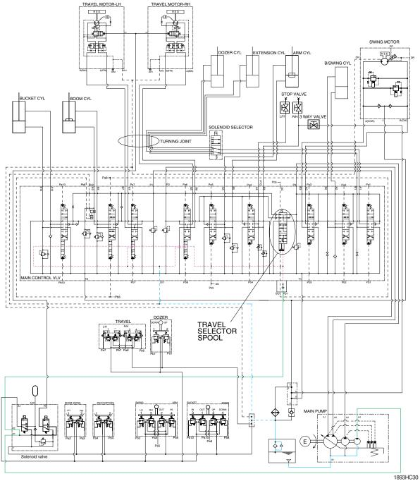
The oil from the A1, A2, A3 pump flows through the neutral oil passage, bypass oil passage and confluence oil passage in the main control valve. Then the oil goes to each actuator and operates them. Check valves and orifices are located on these oil passage in the main control valve. These control the oil from the main pumps so as to correspond to the operation of each actuator and smooth the combined operation.
