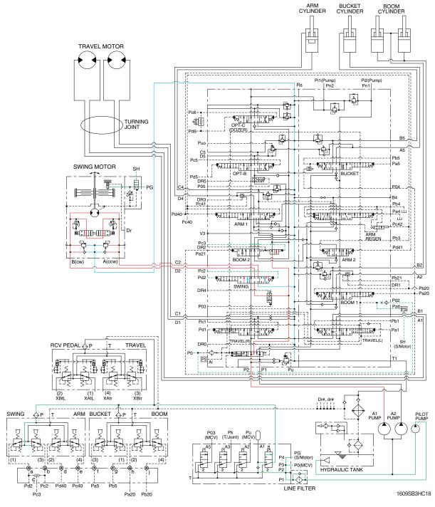
When the left control lever is pushed left or right, the swing spool in the main control valve is moved to the left or right swing position by the pilot oil pressure from the remote control valve.
