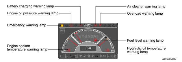
\* Each warning lamp on the top of the LCD pops up on the center of LCD and the buzzer sounds when the each warning is happened. The pop-up warning lamp moves to the original position and blinks when the select switch is pushed. And the buzzer stops. Refer to page 5-34 for the select switch.
