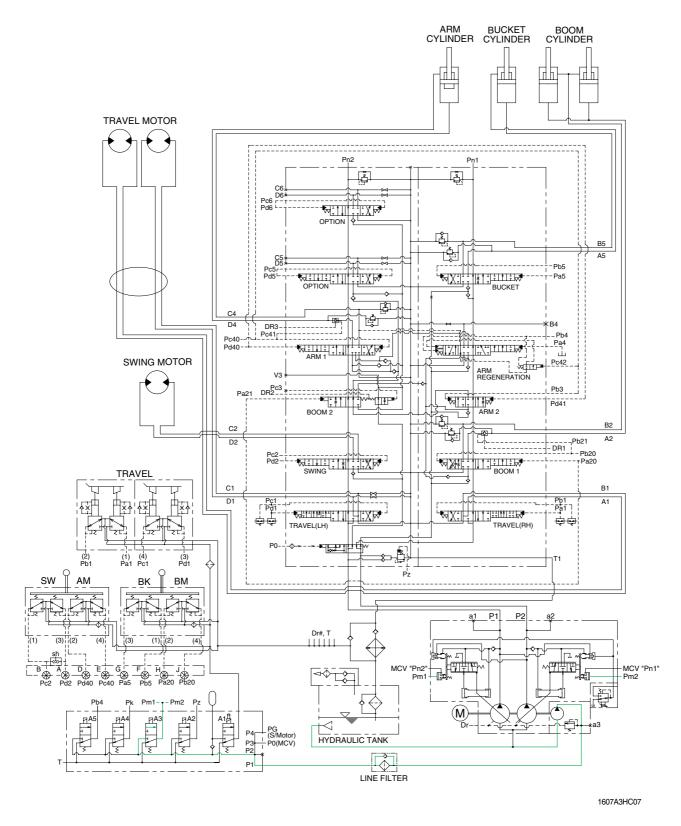
When the breaker operation mode is selected on the cluster, max flow cut off solenoid valve actuates automatically.
