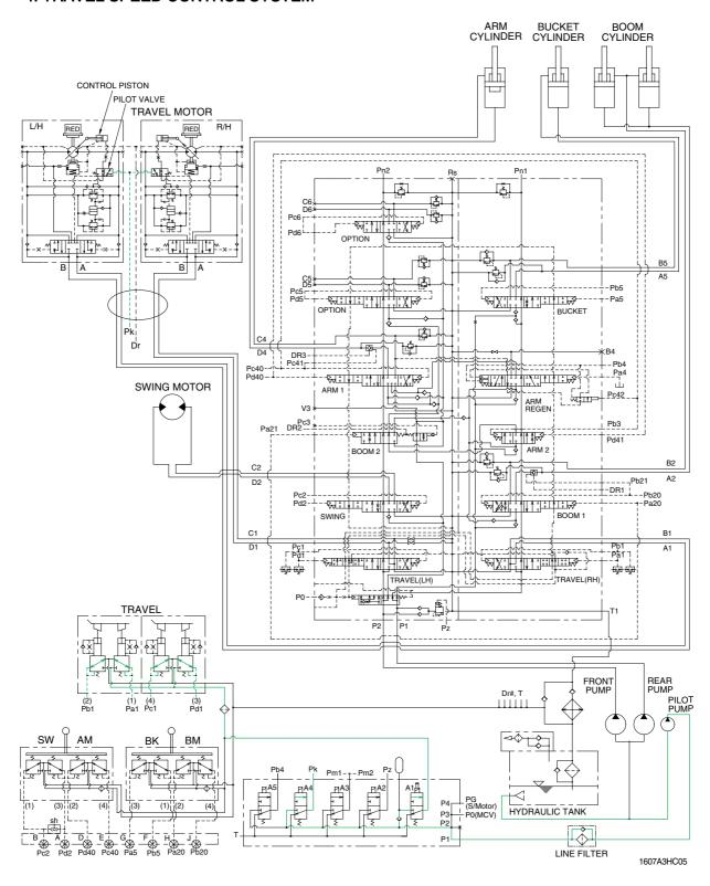
When the travel speed switch is pushed, the travel speed solenoid valve is actuated and the discharged oil from the pilot pump flows to the Pk port of pilot valve in the travel motors. As a result, the control piston is pushed by the main oil flow, thus the displacement is minimized. When the travel speed switch is pushed once more, the travel speed solenoid valve is return to original position by the force of spring, the hydraulic oil of Pk port returns to the hydraulic tank.
