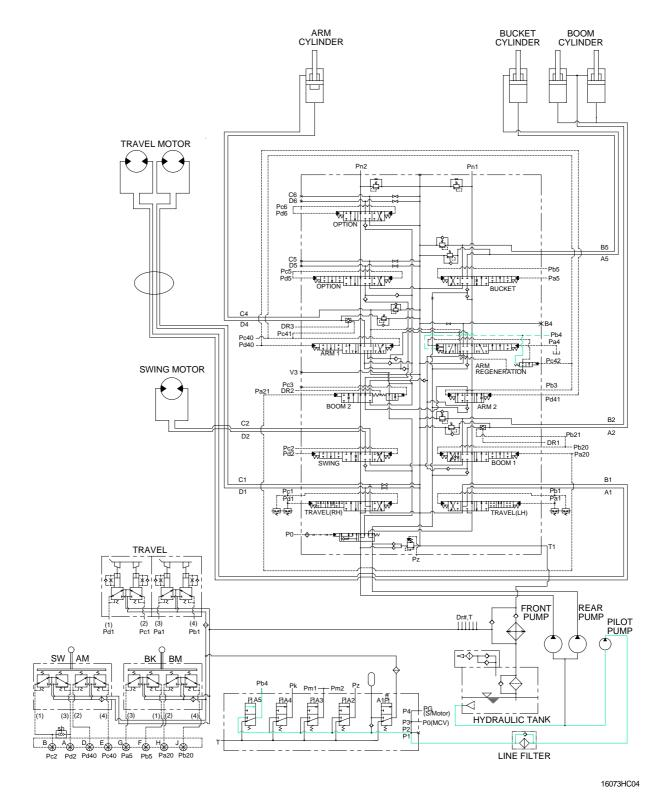
Then the heavy duty mode switch on the cluster is pushed ON, the arm regeneration solenoid valve is deactivated and the arm regeneration spool is returned to neutral position.
