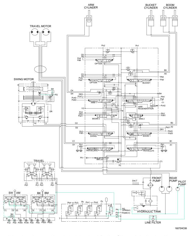
When the swing control lever is tilted, the pilot oil flow into SH port of shuttle valve, this pressure move spool so, discharged oil from pilot valve flow into PG port.
